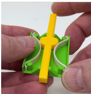
Figure 57. Snap action mechanism (from https://www.youtube.com/watch?v=sG_mKVGgQf0 )
