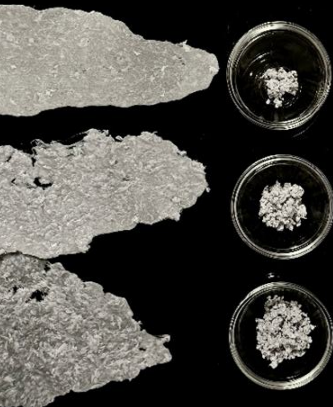
Figure 6. PCL and different amounts of paper pulp blends
