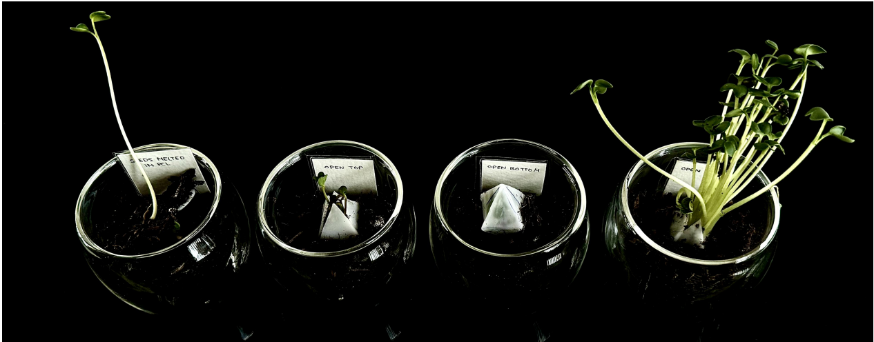
Figure 17. Radish seeds in various PCL capsules after one week. 1) Seeds melted into PCL. 2) Seeds in capsule with open top. 3) Seeds in capsule with open bottom. 4) Seeds in capsule with open top and bottom
