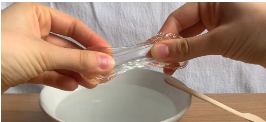
Figure 1. Molding heated PCL
