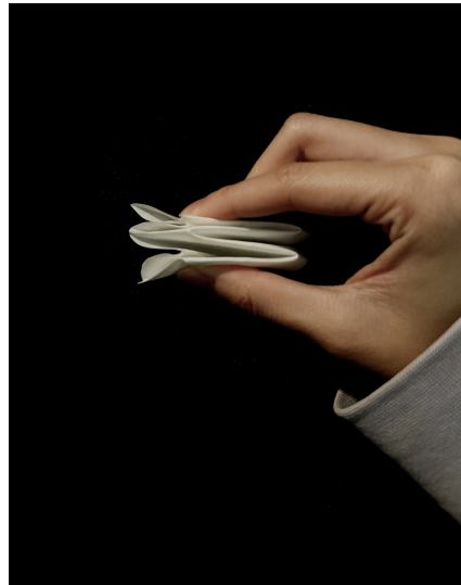
Figure 10. Bistable PCL origami structure
